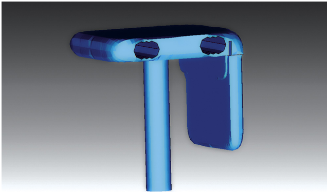
Figure 1. Predesign of film holder with 2 perpendicular plates (occlusal plate and imaging plate), guide post, and clip.
